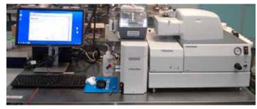
**S3500 MICROTRAC** with image analysis to monitor particle size and morphology
