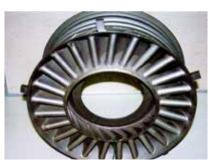
JET ENGINE NOZZLE ASSEMBLY NICROBRAZ® 125 BNi-1
