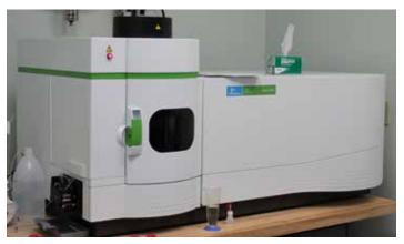
ICP SPECTROMETER to analyze chemical compositions of all alloys
