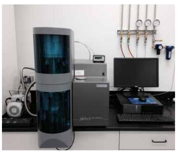
THERMAL ANALYZER (DSC/DTA/TGA) to measure solidus and liquidus temperature
